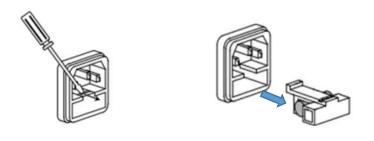
Remove and insert the proper fuse into the fuse holder.
